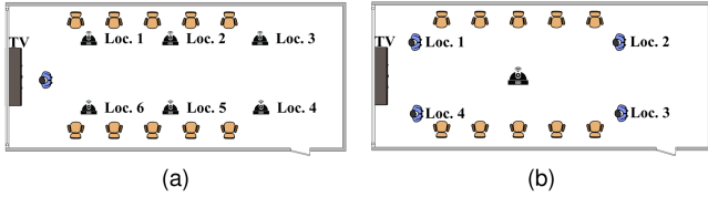
Fig. 11. (a) Different locations of the transmitter (i.e., a camera) and (b) different locations of the subject in Room 1.
